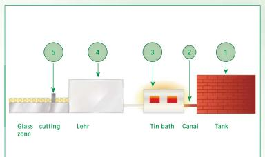
Different pyrometer models are used in the industrial floatglass production as the temperature of molten glass as well as solid glass have to be determined.
