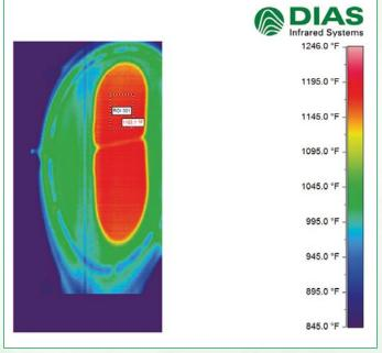
The PYROLINE camera is placed just out of view at the top of the image above. It is positioned to look down at the hoop and glass as it leaves the furnace. The line speed on the camera is set to 256 Hz, with the line oriented perpendicular to the direction of travel of the rotary arm.
