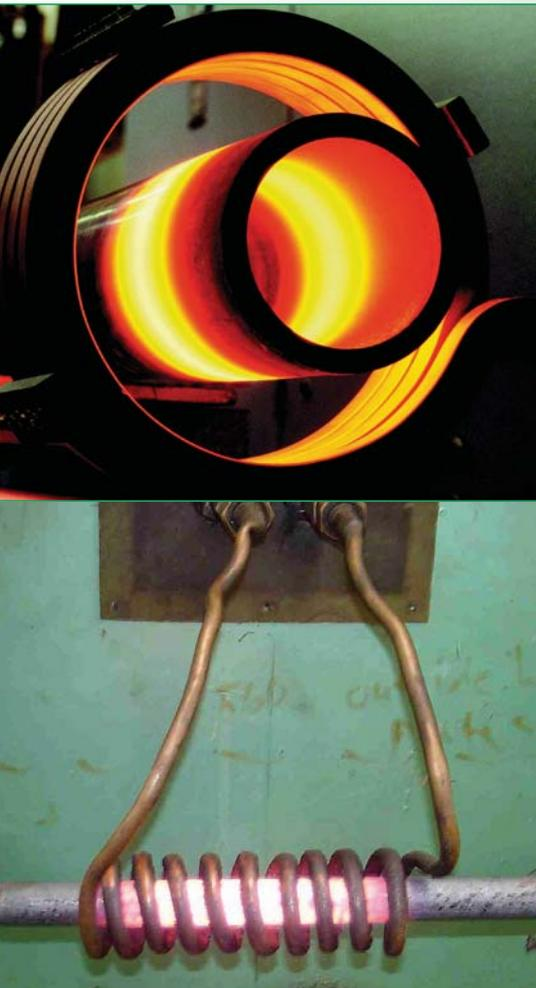
The inductive hardening is a heat treatment for surface hardening, mainly used for complicated shaped workpieces or for partially hardening of specific parts of an item. One of the most important parameters at induction hardening is the correct temperature of the item to guarantee the required quality of the product. This temperature is approximately 900 °C depending on the material.
