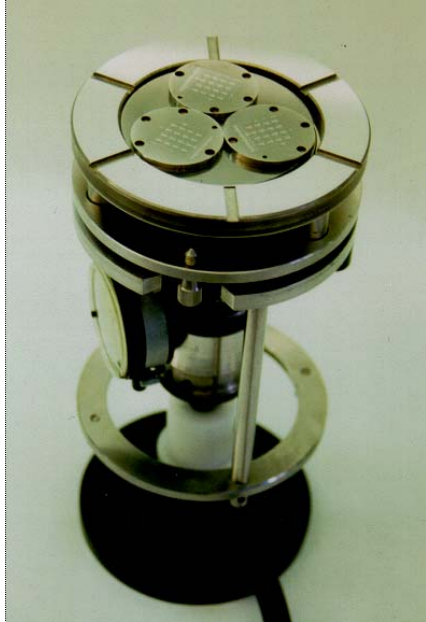
Figure 4: Polishing jig with \text{LiTaO}_3 -samples
