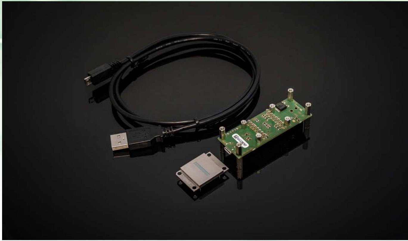
The **Evaluation Kit** allows easy operation of the PYROSENS arrays. It consists of a small circuit board with complete electronics and software by which the electronics is controlled via USB connection from a Windows PC. The power can be provided by the USB port or a separate power supply (9 V). For synchronisation with further external components, such as for radiation modulation, a trigger pulse is provided.
