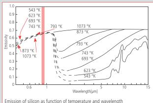
Emission of silicon as function of temperature and wavelength Quelle: Sato, T., Jap., Appl. Phys. 6, March, 1967, p. 339-347
