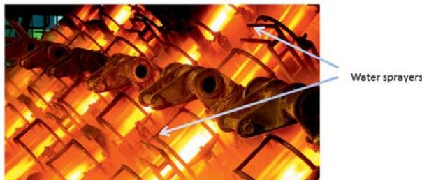
Fig. 2. Continuous casting (control of the secondary cooling)
